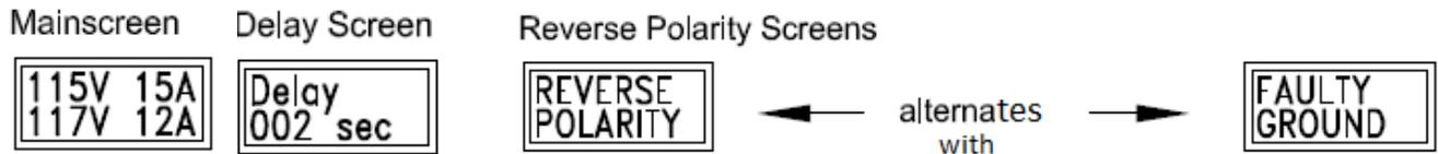
**L1 VOLT and L2 VOLT Screens** - These screens are useful for viewing the line voltages when the Main Screen is in Delay or when it shows that L1 or L2 have a fault such as a line voltage that is too low or too high. The Main Screen will display the line voltage if it is between 102 and 132 volts; otherwise it will show that the line has a fault. The L1 VOLT and L2 VOLT screens however display a greater range, from 90 to 140Volts. The L2 VOLT screen is only shown when using a 50Amp Surge Guard.
